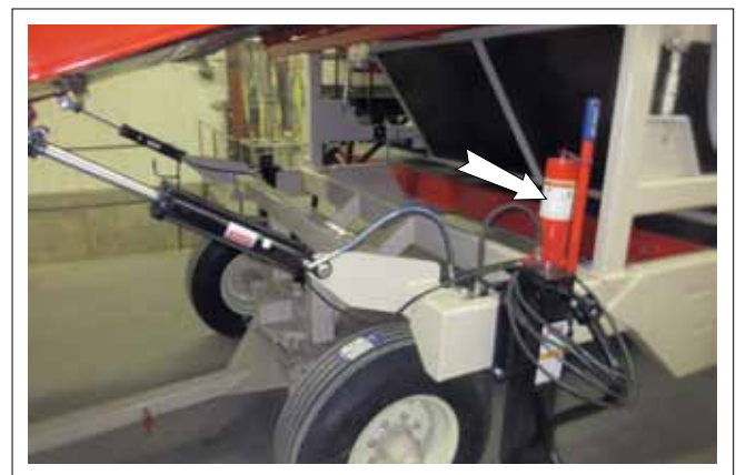
FIG. 8 HOPPER POSITION JACK CONTROL LEVER
