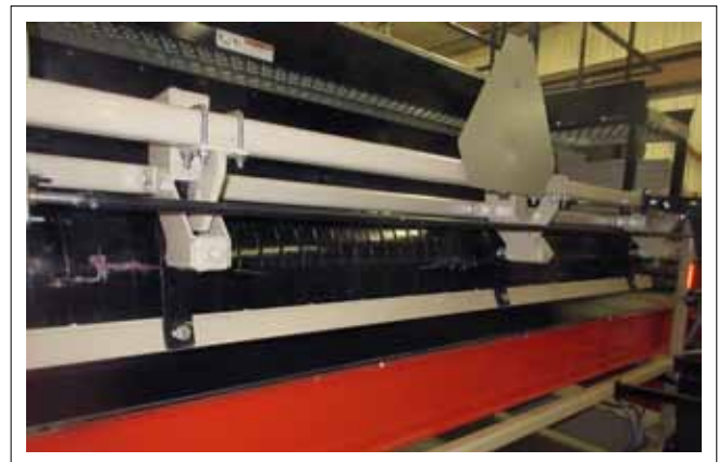
FIG. 30 LARGE POTATO ROLL SCRAPERS (TYPICAL)
