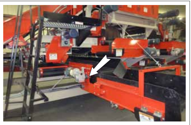
FIG. 41 DISCHARGE CONVEYOR PIVOTS (TYPICAL)
