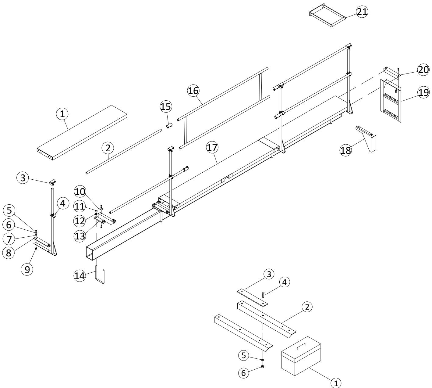
**Front Seed Tank Platform with Removable Center Handrail**
