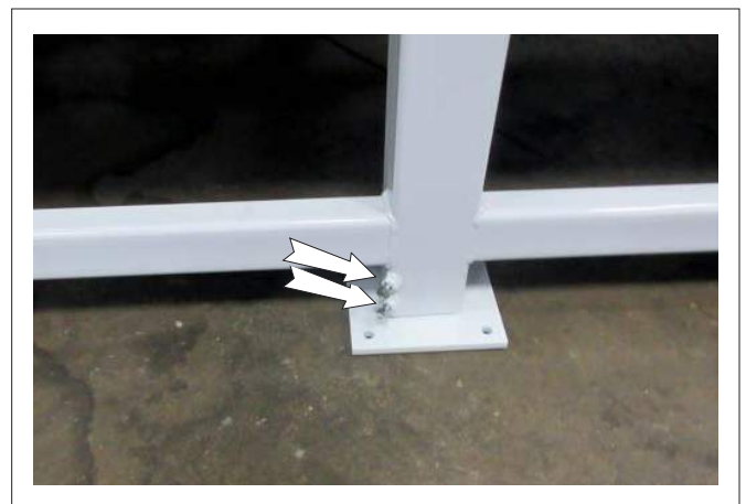
FIG. 9 FEET FRAME SET SCREWS (TYPICAL)
