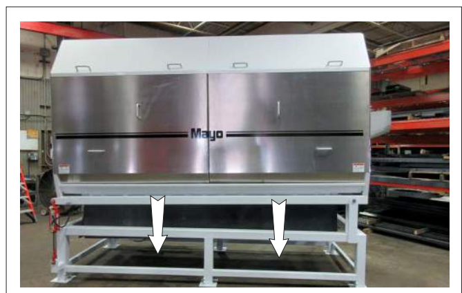
FIG. 22 WATER CONTAINMENT AREA
