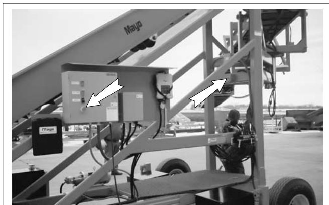
Master Control Panel / Frame
